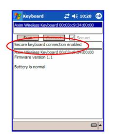
12. If the connection process is successful, the Secure keyboard connection enabled message will display on the Pocket PC device. This is the normal mode for wireless communication between the Axim<sup>™</sup> Wireless keyboard and the Pocket PC device during use.
